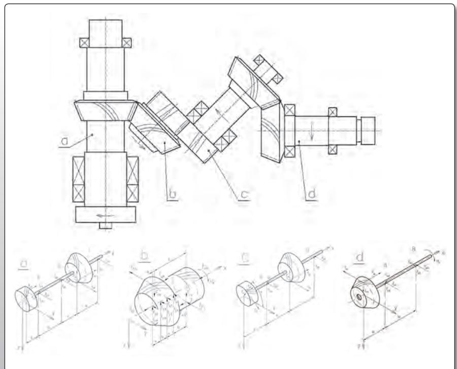
Fig. 1.6.2: Force equilibrium on milling head shafts
