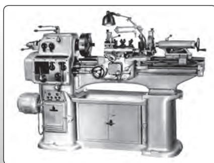
Fig. 1.9.8: Original appearance of the centre lathe made by TOS Čelákovice at the end of the fifties
