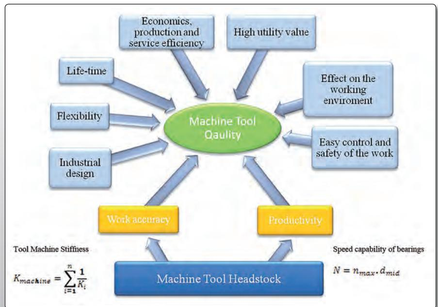
Fig. 3.2.1: Influence of the main factors on the machine tool quality
