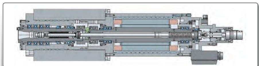
Fig. 3.2.7 Headstock milling machines with clamping system [SKF]
