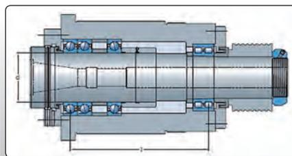
Fig. 3.2.3: Tube shape of the headstock body [SKF]
