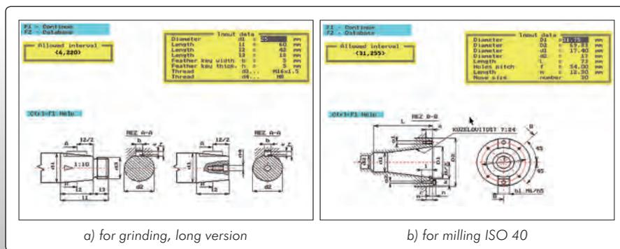
Fig. 3.2.6 The ends of the spindles grinders and milling machines [Javorčík 1991]
