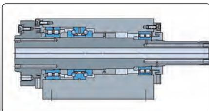
Fig. 3.2.2: Box shape of the headstock body [SKF]
