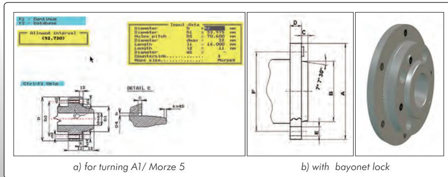
Fig. 3.2.5 The ends of the spindle lathes [Javorčík 1991]
