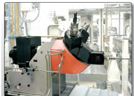
Fig. 3.5.10: Example of the turret in the crown type used at the machine [Sauter]
