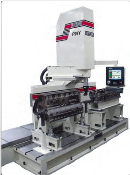
Fig. 3.6.4: Principle of the doubled workplace [Rottler USA]
