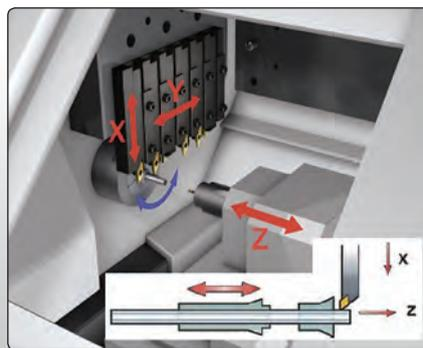
Fig. 3.6.6: Workpiece exchange principle at long rotative automatic machines [Sandvik Coromant]
