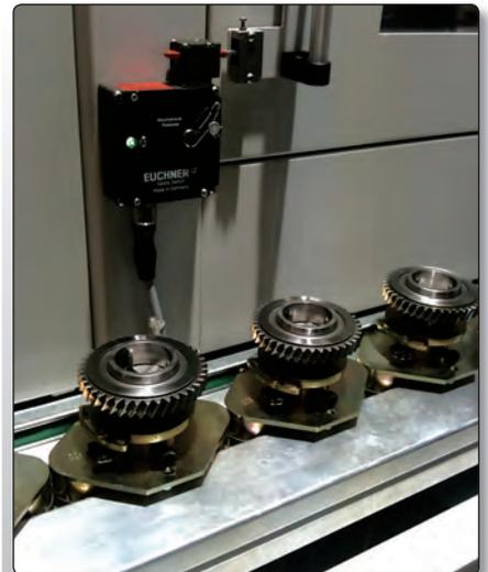
Fig. 3.6.9: Carrying plate for rotary workpieces [MAG]
