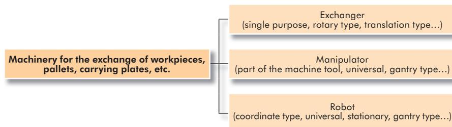
Fig. 3.6.2: Equipment for the automatic workpiece exchange
