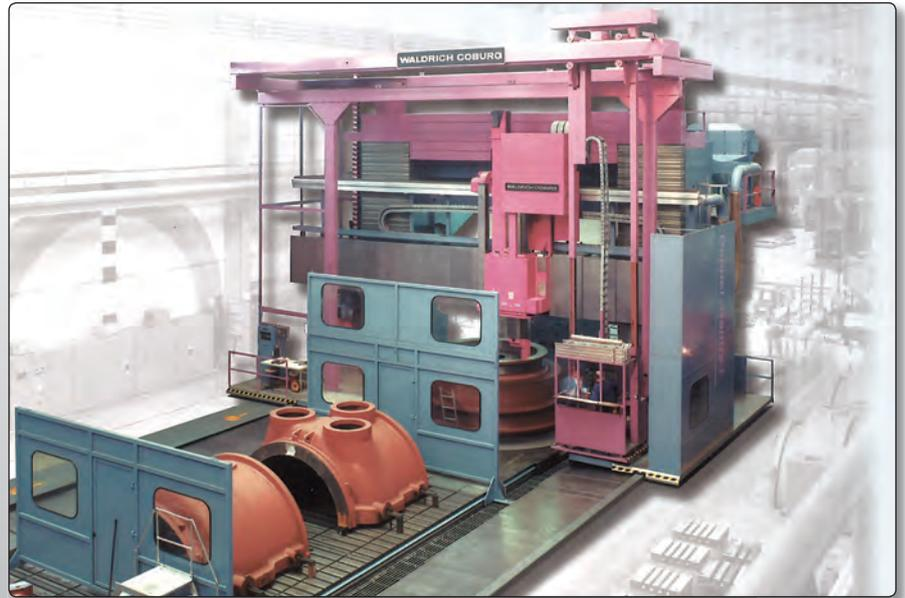
Fig. 3.6.5: Machining a setting of more workpieces on one machine [Waldrich-Coburg]
