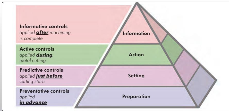
Fig. 3.8.1: Productive process pyramid [Renishaw]
