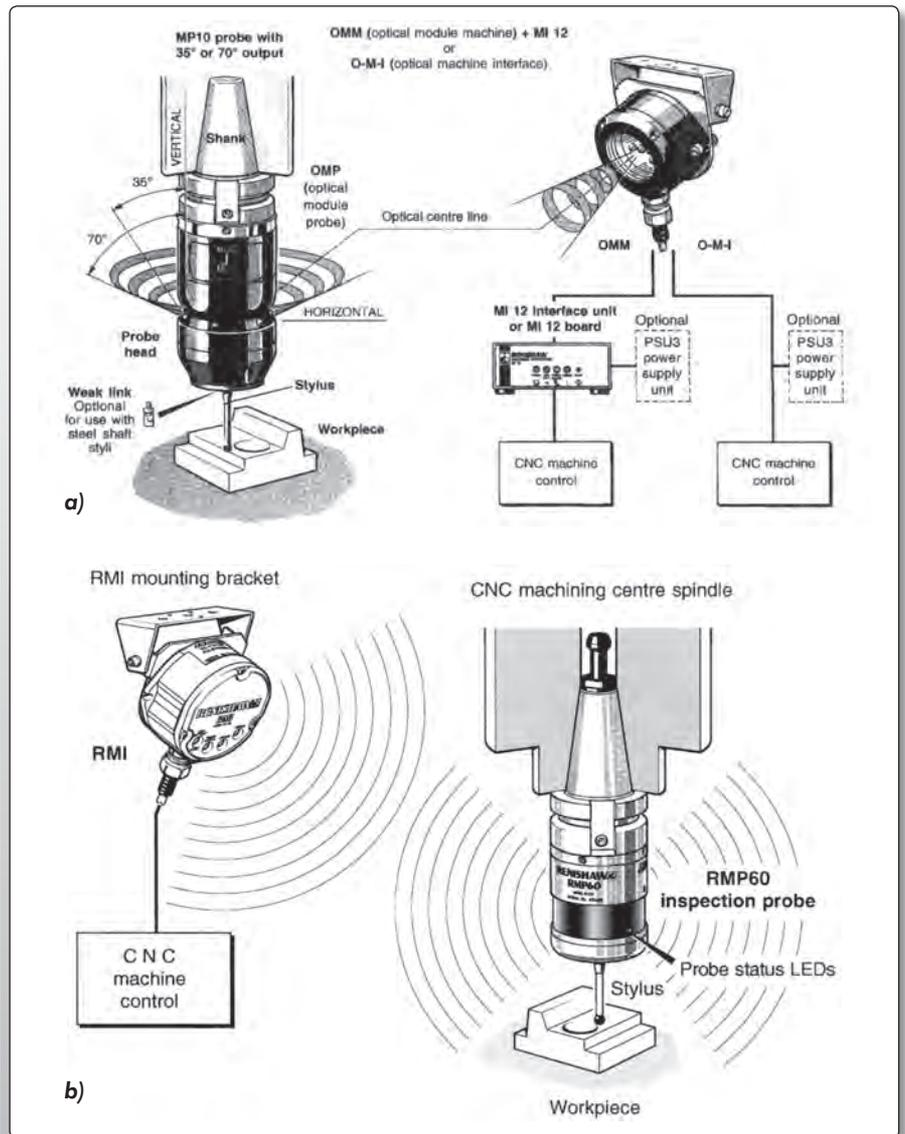
Fig. 3.8.7: Workpiece measuring probes – a) optical transfer, b) radio transfer [Renishaw]
