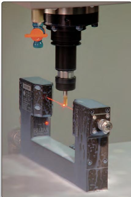
Fig. 3.8.6: Measuring mechanism of the tool measuring probe with laser signal generation [Blum]
