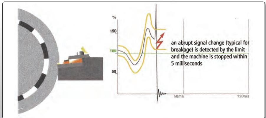
Fig. 3.8.3: Measuring example of the turning cutting process [Prometec]
