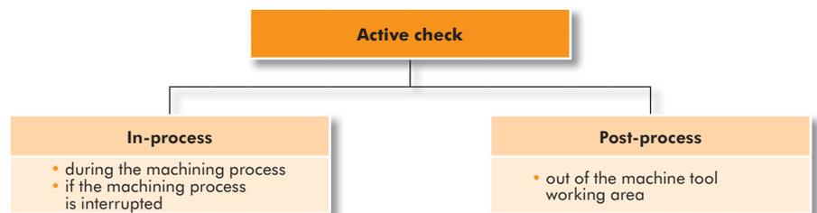
Fig. 3.8.2: Types of the active check at the CNC machine tool
