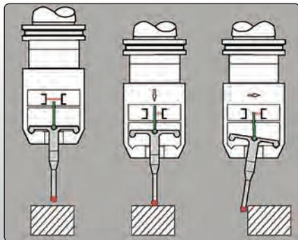
Fig. 3.8.5: Measuring mechanism of the workpiece measuring probe with optoelectronic signal generation [Blum]
