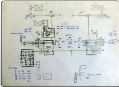
Fig. 4.3.5: Functional elaboration of the motion groups at the MCSY machine [Borkovec]
