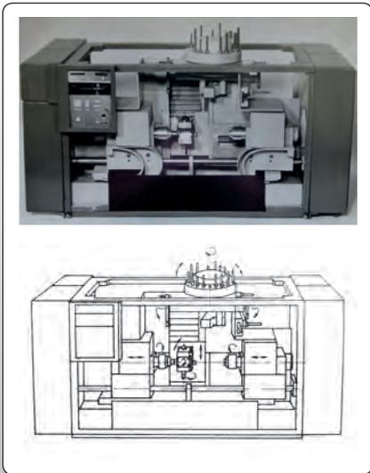
Fig. 4.3.6: Wooden model of the MSCY machine and its kinematic diagram [Borkovec]
