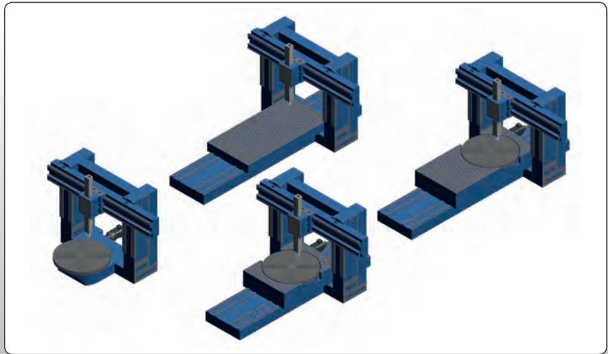
Fig. 4.3.1: Kinematic adaptability of multifunctional machining centres [Toshulin]
