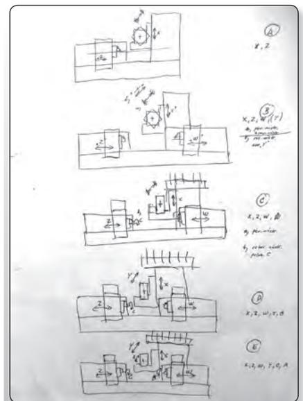
Fig. 4.3.4: Elaboration of the unit-built system of the MCSY machine new solution [Borkovec]
