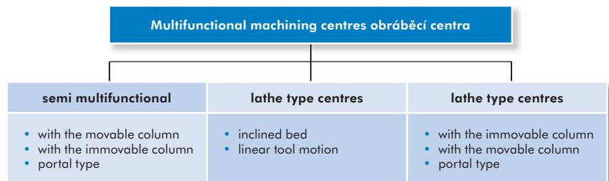
Fig. 4.3.2: Division of the multifunctional machining centres
