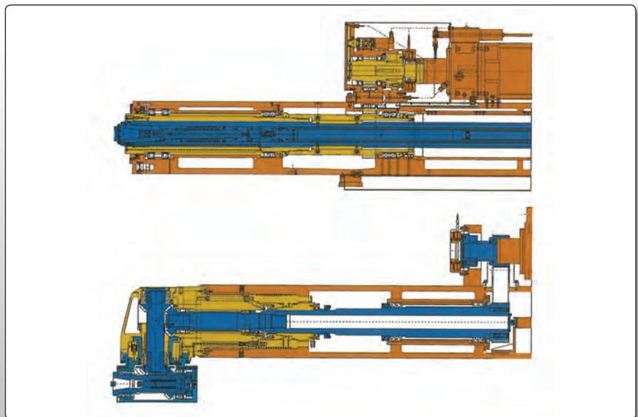
Fig. 5.4.10: Example of the rotary tool drive and of the tailstock sleeve at the horizontal boring and milling machine [Škoda Machine Tool]
