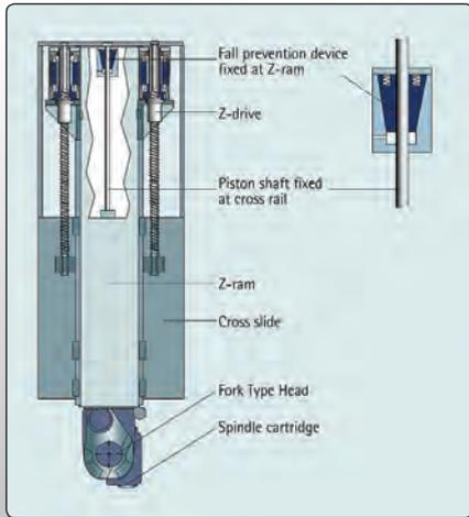
Fig. 5.4.7: Example of the ram safety brake [DST]
