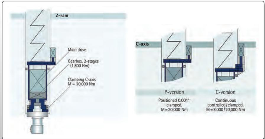
Fig. 5.4.8: Rams having big cross sections can be equipped with the C axis [DST]
