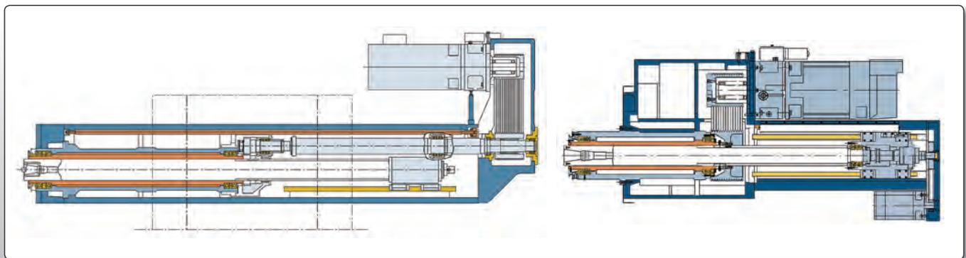
Fig. 5.4.11: Drive kinematics of the ram and of the headstock [Union]
