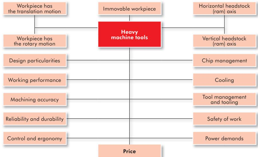
Fig. 5.4.1: Heavy machine tools and their specific features
