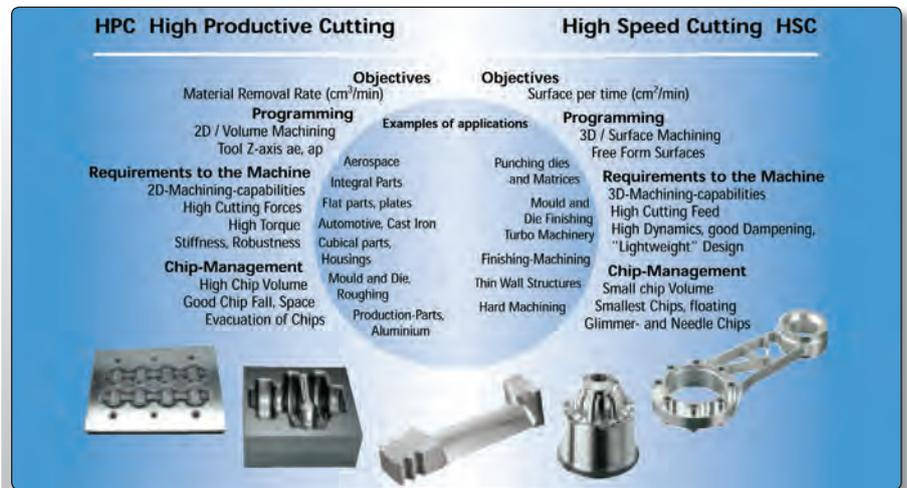
Fig. 5.5.2: Comparison of two main technological trends at High Performance Cutting [Mikron]
