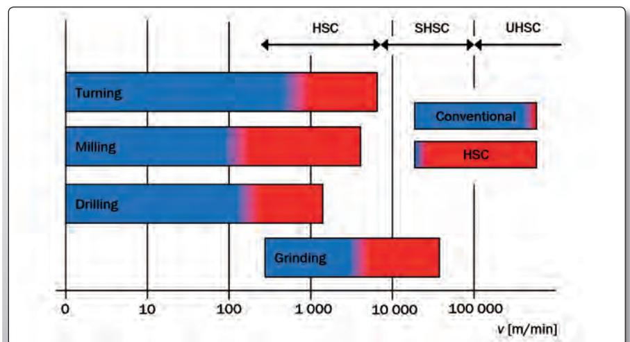
Fig. 5.5.7: Manufacturing technologies and used cutting speeds
