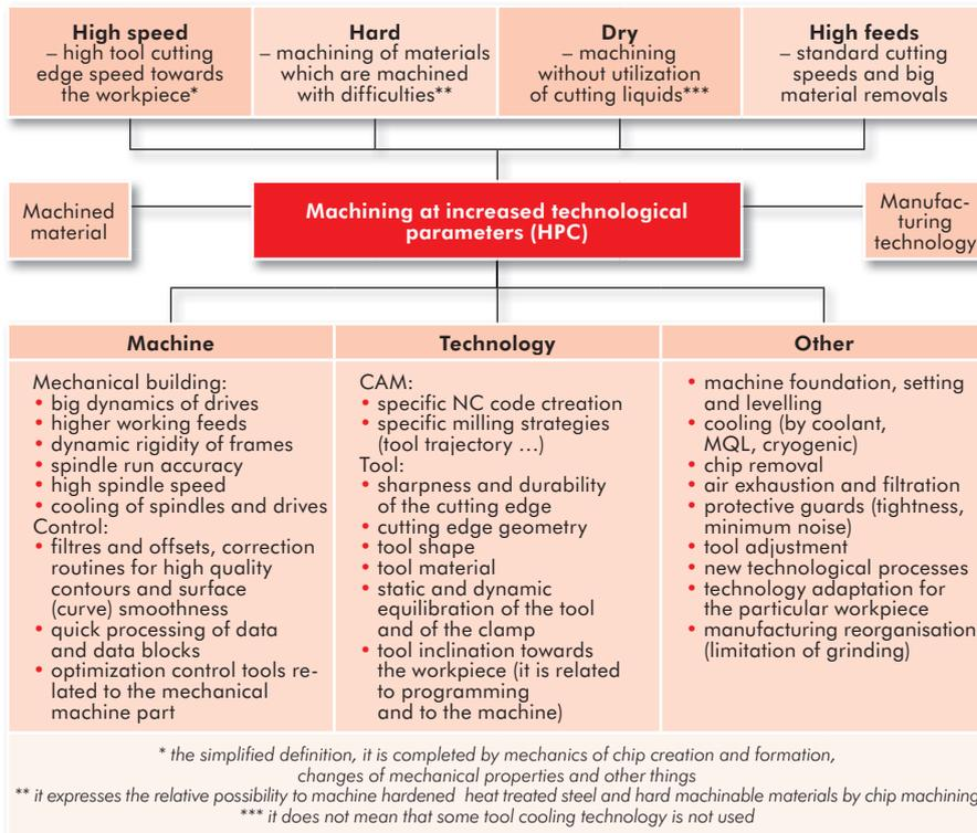
Fig. 5.5.1: Machining at the increased technological parameters – High Performance Cutting
