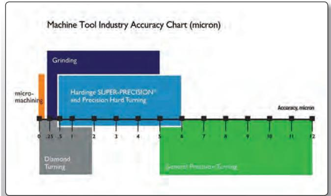
Fig. 5.5.4: HSC technologies replace grinding [Hardinge]
