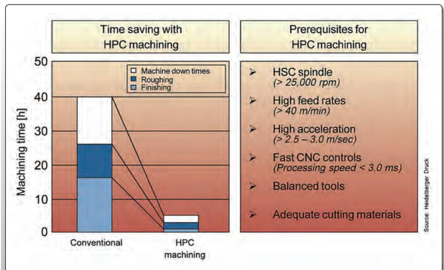
Fig. 5.5.8: Example how to increase productivity using HPC [Ceratizit]
