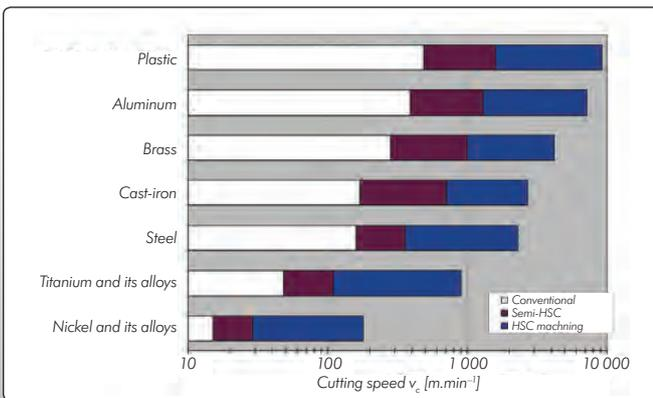
Fig. 5.5.5: Speed ranges of HSC technologies according to Walter company [Walter]
