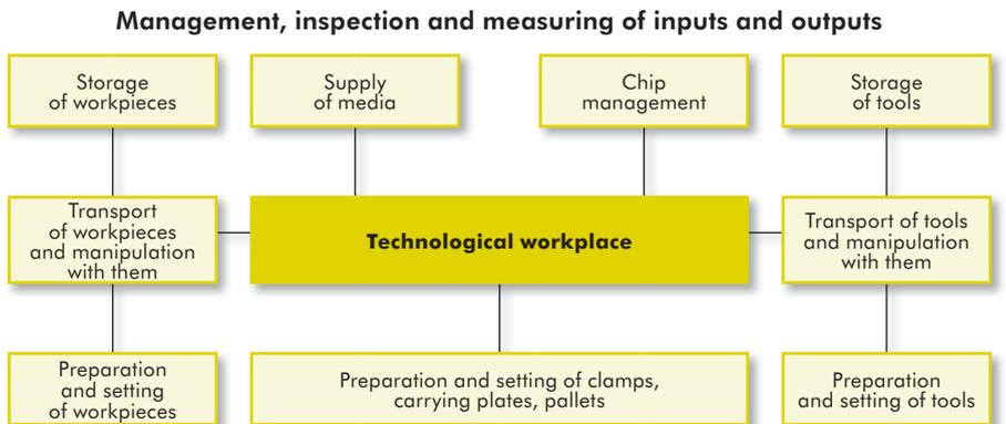
Fig. 6.1.1: Structure of the automatized production systems (AVS)
