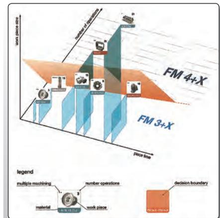
Fig. 6.1.3: Manufacturing time, the number of operations and the workpiece size serve to choose the manufacturing machinery [Elha]
