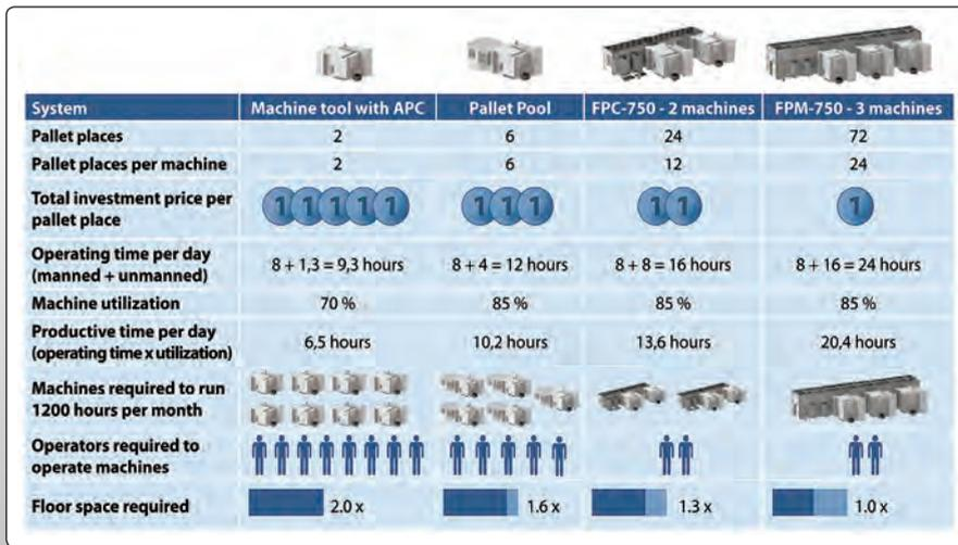
Fig. 6.1.6: Benefits of transition from the machine having two pallets to the more sophisticated automation ways [Fastems]
