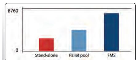
Fig. 6.1.4: Working productivity of the automatized production system expressed by the number of spindle operating hours [Fastems]
