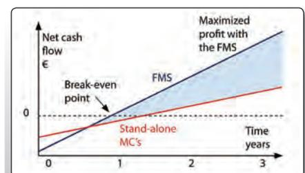
Fig. 6.1.5: Economic justification of the automatized production system [Fastems]
