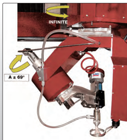
Fig. 6.3.8: Cutting head [WaterJet]
