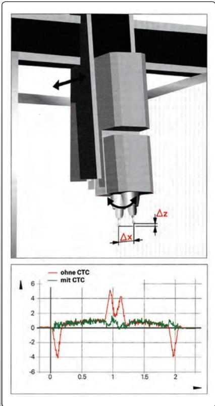
Fig. 7.2.5: Keeping the tool position setting error in the tolerance thanks to the CTC function [Heidenhain]
