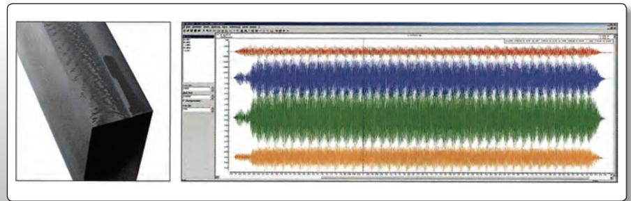
Fig. 7.2.3: Oscillation consequences on the workpiece surface [Heidenhain]
