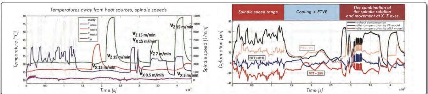
Fig. 7.2.6: Course of speed and feed velocities, including the result comparison of the transmission function and MLR temperature compensation [Kovosvit MAS and Engineering Faculty of Czech Technical University in Prague]
