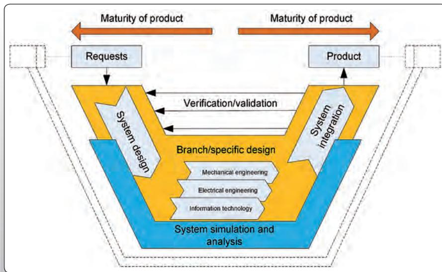
Fig. 7.3.3: V-model of the mechatronic system design process [VDI 2004]
