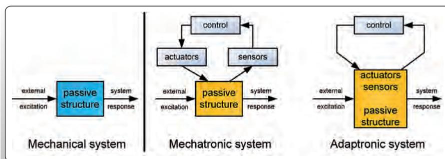
Fig. 7.3.1: Characteristics of the mechatronic systems
