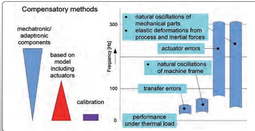
Fig. 7.3.2: Error zone width of the machine tool and possibilities how to correct errors [Neugebauer 2007]
