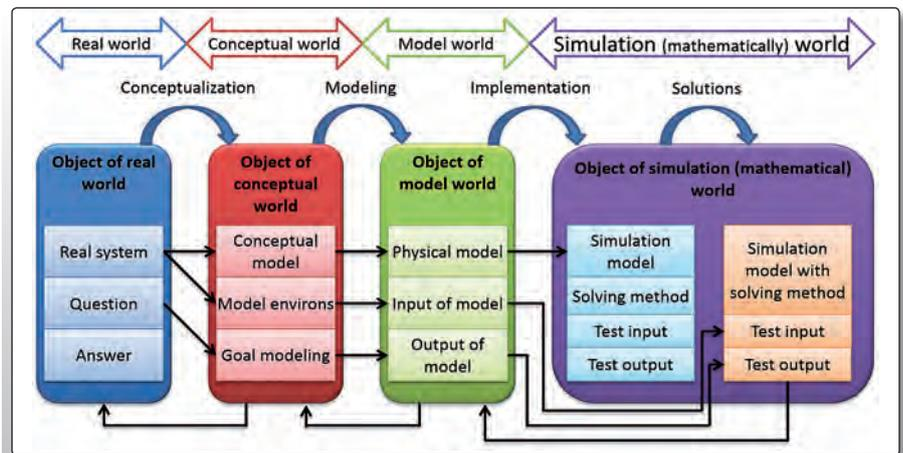
Fig. 8.3.3: Planning of the simulation modeling of a technical system
