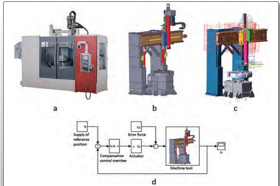
Fig. 8.3.2: Transformation of a real machine into an idealized model of reality; a - real machine, b – conceptual model, c --physical model, d – computer simulation
