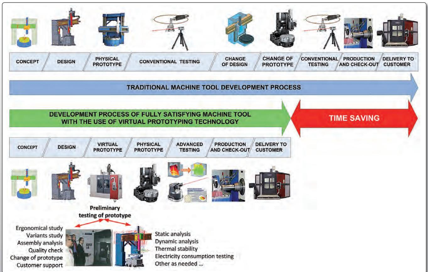
Fig. 8.3.1: Comparison of the traditional process of development of a machine tool with that applying virtual prototyping
