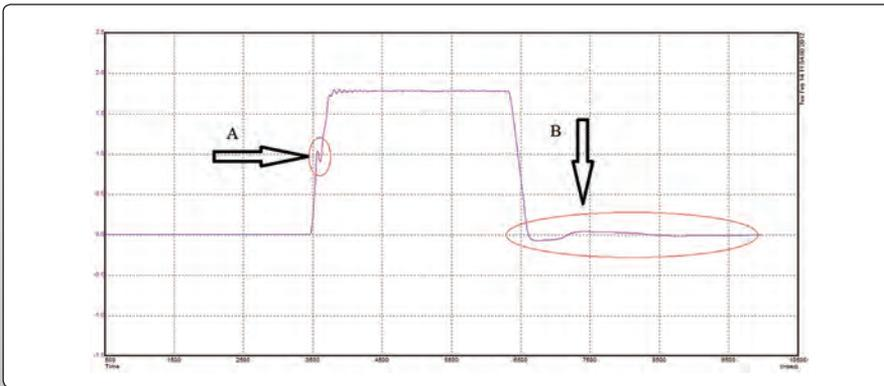
Fig. 9.2.4: Graphical course of the position deviation at a jump change [Fermat]
