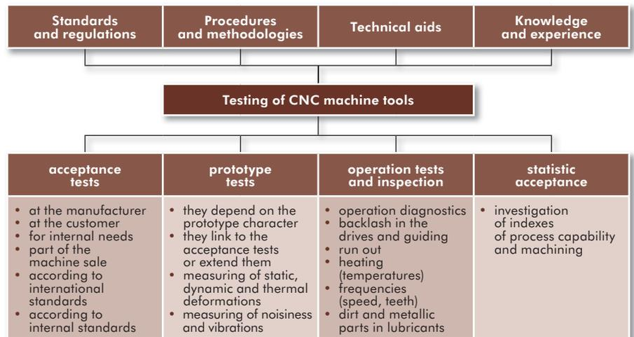
Fig. 9.3.1: Testing of CNC machine tools
