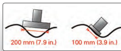
Fig. 9.3.8: Influence of the measuring instrument base size on the measuring accuracy [Dixi Machines]
