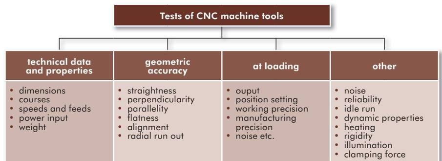
Fig. 9.3.2: Acceptance tests of machine tools
