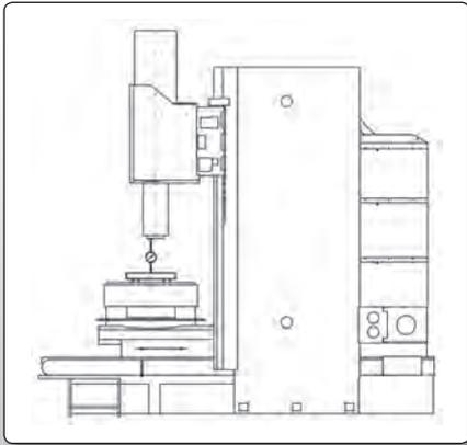
Fig. 9.3.6: Example of measuring of the rectilinear motion of the slide with the technological pallet in the Y axis in the horizontal plane [Toshulin]
