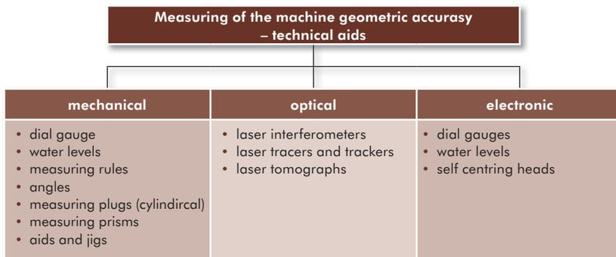
Fig. 9.3.4: Overview of technical aids specified to measure the machine geometric accuracy
