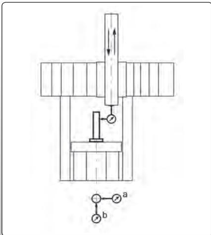
Fig. 9.3.7: Example of measuring of the radial run out of the inside cone in the straight head [Toshulin]
