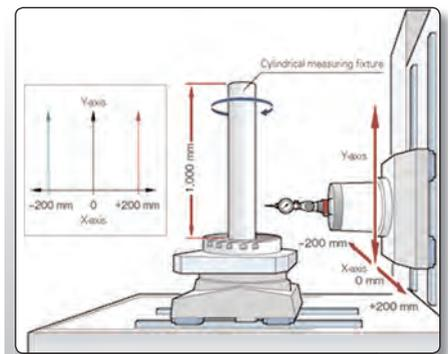
Fig. 9.3.5: Measuring of the accuracy (straightness) of the Y axis [Dixi Machines]
